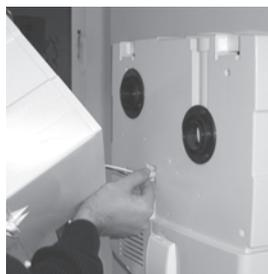
3. Fasten the connector of the weak current wire to the counter piece of the filter unit. The connector of the weak current wire can be found separately in the package.
