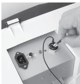
9. Fasten the weak current wires and the mains cable to the circuit board of the machine.
