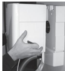
4. Push the central unit directly towards the filter unit. Push the central unit toward the filter unit.
