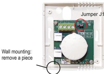
TMR/SP sensor is placed at the height of approximately 150 cm in a place where it measures the mean temperature of the premises. Do not place the room sensor on direct sunlight or close to a heat source.
